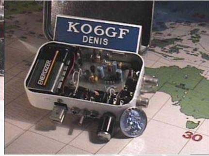
• Simple 250mW transceiver kit from HSC Electronics
