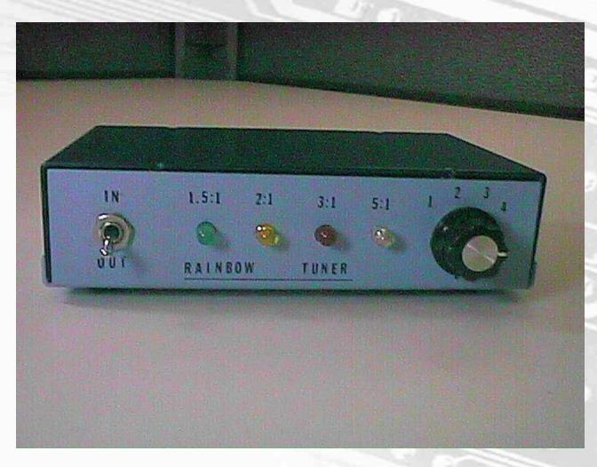
• Custom enclosure with panel mounted switch for tuner inductor settings
