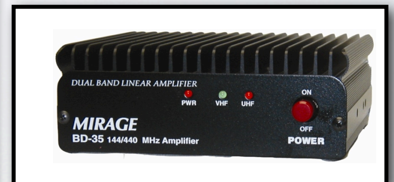
Dual Band Amplifier 5 watts In 35 watts Out
